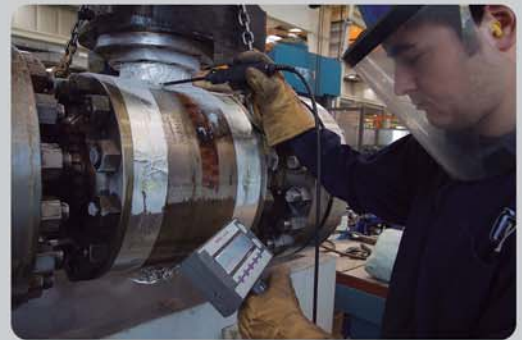
Fugitive Emission Test in prototype
