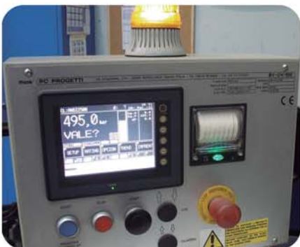
Computer operated pressure test bench
