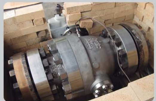
Fire-Safe Test in prototype
